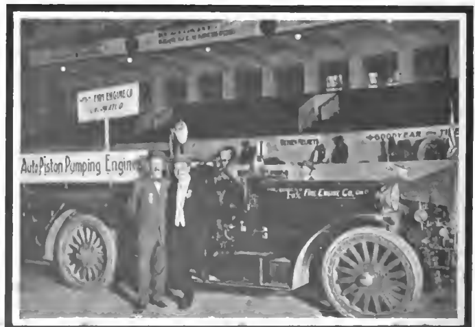
Ahrens-Fox pumping engine with pump located in front of radiator
